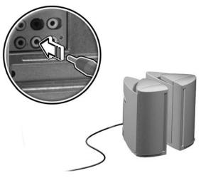
• Audio line-in device: Connects to the audio-in/line-in jack (()) (light blue jack) located on the rear panel of your computer
